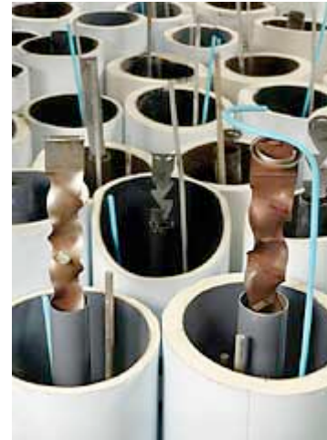
COVERAGE COMPARED A look inside these gas water heaters confirms that a move up in warranty coverage from 6 years (foreground, left) to 12 years (foreground, right) typically buys thicker outer heat insulation, among other features.
